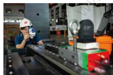
The photoelectric autocollimator check I
