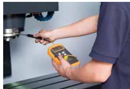
The spindle temperature detecting
