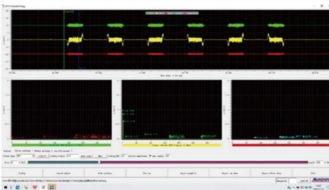
Vibration frequency and amplitude when making G00 movement on Z axis
