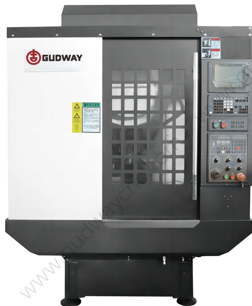
■ GLV-500 table size(X*Y-axis):650x400mm
